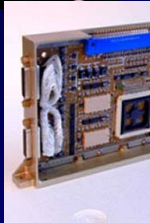
CCSDS TMTC digital module for the CNES micro- satellites
